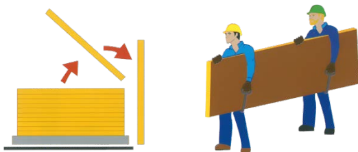
Figure 3 Handling equipment as well as gloves must be clean and such not to damage the items.
